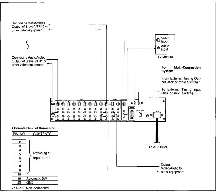
Connect each set of Input Terminals to the Audio/Video Output of video equipment.
